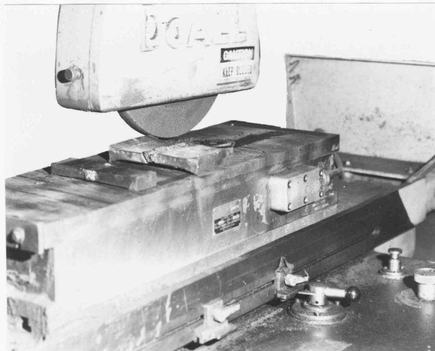
Figure 3.8. Grinding the Welded Plate
